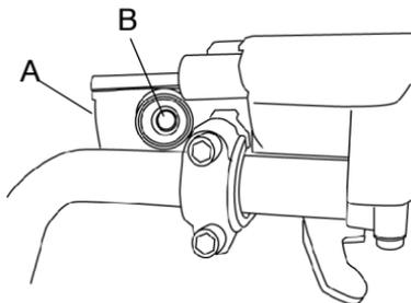
**NOTE:** When checking the fluid level, position the ATV on level ground with the handlebars turned so the top of the reservoir is level. If the fluid level is low, add DOT 3 brake fluid. **DO NOT OVERFILL.** See page 103 for the part numbers of Polaris products.
