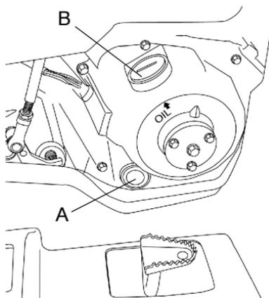
3. Remove the fill plug (B) and add the recommended oil as needed.
