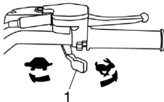
This ATV is equipped with Polaris Electronic Throttle Control (ETC), which is designed to reduce the risk of a frozen or stuck throttle. If the throttle cable should stick in an open position when the operator releases the throttle lever, the engine will stop, and power to the rear wheels will cease.
