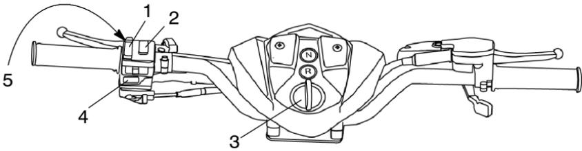
1. **Light Switch/Hi-Lo Beam Control** - The lights won't turn on unless the main key switch is on.
