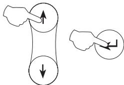
6. Press the  $\leftarrow$  button to enter the CARD or USB, to select the file folder. Press the CALL/HELP button to call the menu, and select the desired files. Press the  $\leftarrow$  button to confirm.
