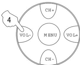
5. Press the VOL+ button to enter the Fine Tune Menu, and then the VOL- button to search downwards or the VOL+ button to search upwards until it has searched the TV signal you need.
