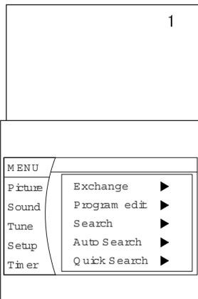
2. Press the MENU button to display the menu, then press CH +/- buttons to select TUNE menu, press VOL+ button to enter.
