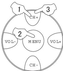
1. Press the CH +/- buttons or Direct select button to select the desired channel number. (For example, the channel 1.)
