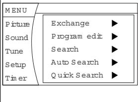
3. Press the CH +/- buttons to move the indicator to "Program edit", then press the VOL+ button to sub-menu.
