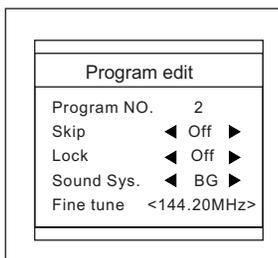
2. Press the VOL+ button to turn the Lock function to "On".
