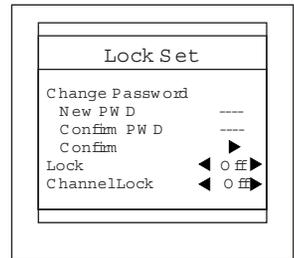
3. Press the CH +/- buttons to move the indicator to "Lock", then press the VOL+ button to turn the function ON or OFF.
