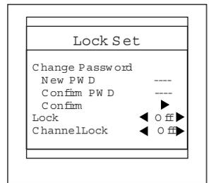
4. Press the CH +/- buttons to move the indicator to "Confirm", and then press the VOL+ to confirm. If it is correct, then the screen displays change successfully.
