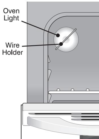
The oven light automatically turns ON when the door is opened. The oven light may also be manually operated by pressing the oven light switch located on top of the control panel. The oven light bulb is located at the rear of the oven and is covered with a glass shield held by a wire holder. The glass shield must be in place whenever the oven is in use.
