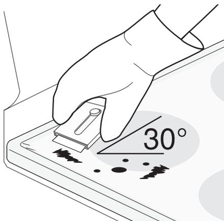
If soils remain, carefully scrape soils with a metal razor blade scraper, holding scraper at a 30 degree angle to the surface. Remove loosened soils with cooktop cleaning cream and buff surface clean.
