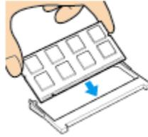
8. Hold the memory module by its edge and push in until it clicks into place as shown in the illustration.
