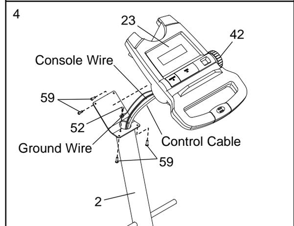
Attach the Console (23) to the Upright (2) with four Console Screws (59). **Be careful to avoid pinching the cable and wires.**
