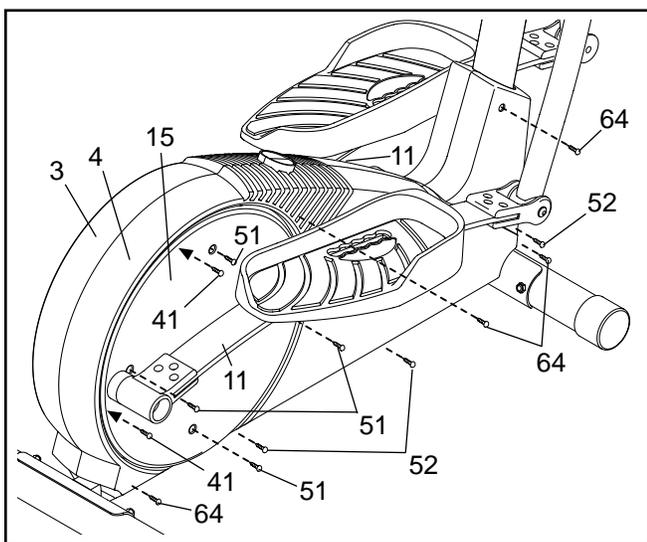
Next, remove the four Screws (51) from the right Pedal Disc (15), and slide the Pedal Disc off. Remove all Screws (52, 64) from the Right Side Shield (4) and the two Bolts (41) from beneath the Pedal Disc, and remove the Right Side Shield (4). Remove all Screws (52) from the Left Side Shield (3), and remove the Left Side Shield.
