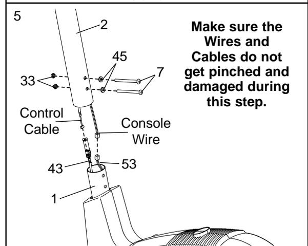
Next, connect the control cable to the Resistance Cable (43) in the following way:
