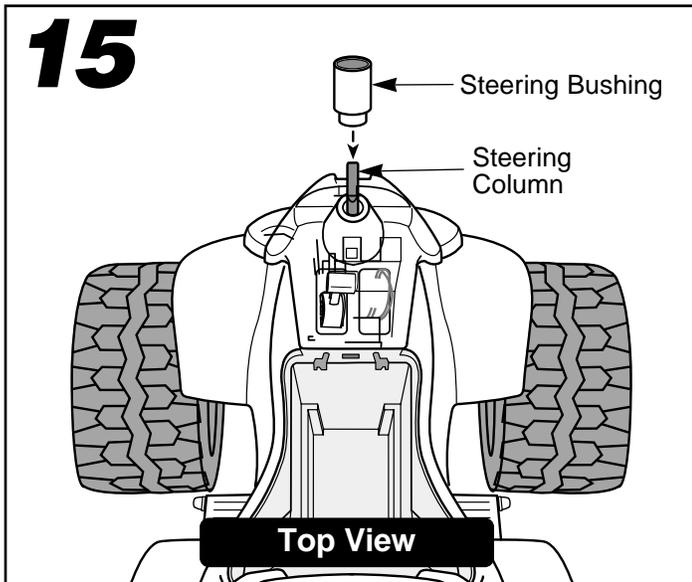
**Hint:** You may want the help of another adult to support the steering column near the steering linkage while assembling the handlebar to the vehicle body.
