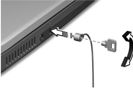
Wrap a computer security lock cable around an immovable object such as a table or locked drawer handle. Insert the lock into the notch and turn the key to secure the lock. Some keyless locks are also available.
