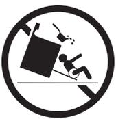
**⚠ WARNING** To reduce the risk of tipping, the range must be secured by properly installed anti-tip bracket provided with the range. To check if the bracket is installed properly, visually check that rear leveling leg is inserted into and fully secured by the anti-tip bracket by removing lower panel or storage drawer. For models with a warmer drawer, grasp the top rear edge of the range and carefully attempt t
