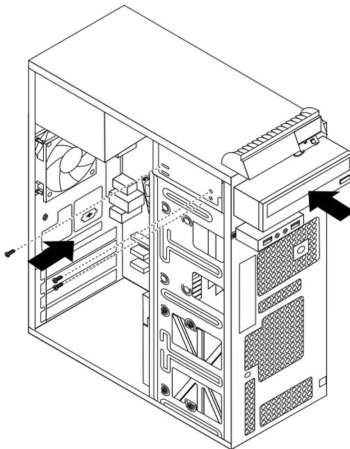
Figure 20. Installing the optical drive
