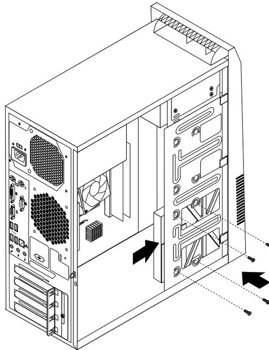
Figure 31. Installing the hard disk drive
