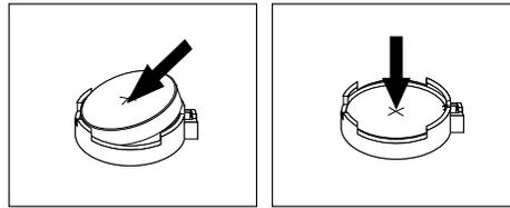
Figure 23. Installing a new battery
