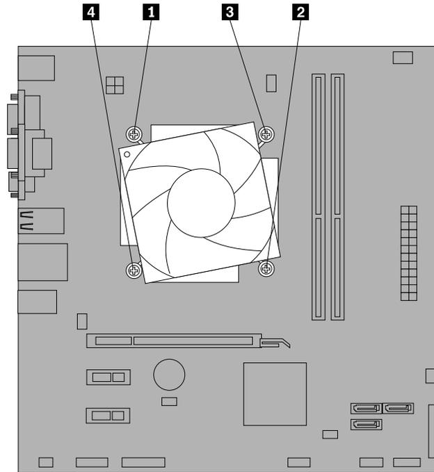
Figure 24. Removing the heat sink and fan assembly
