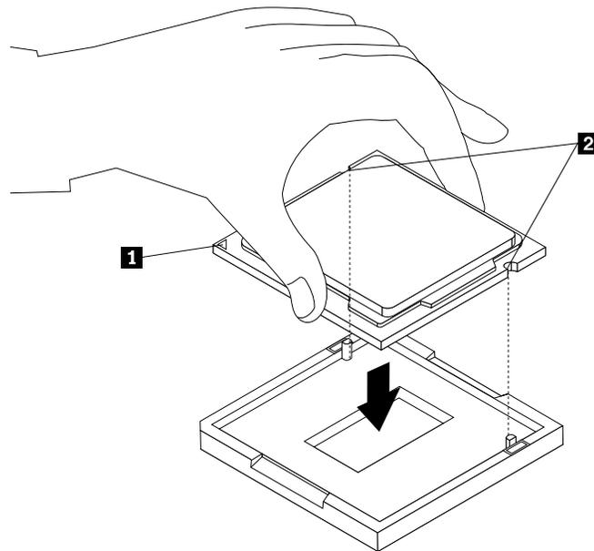
Figure 28. Installing the microprocessor
