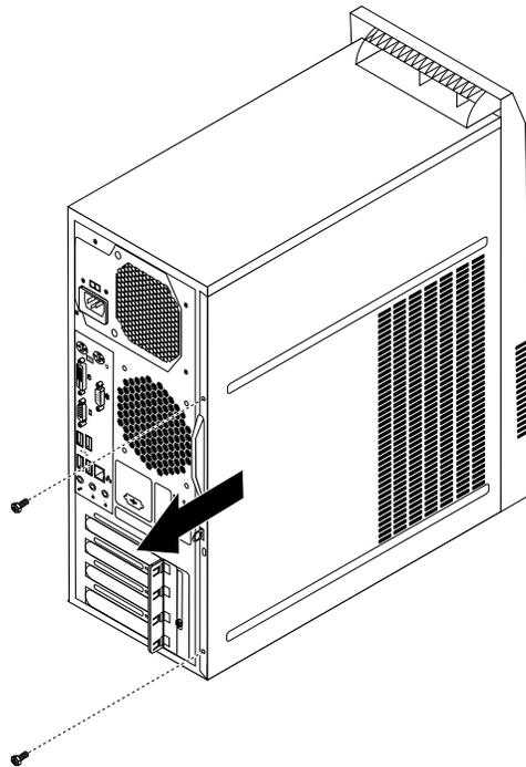
Figure 10. Removing the computer cover
