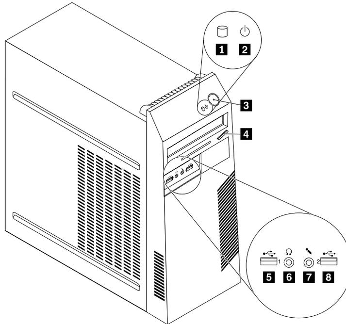
Figure 1. Front connector, control, and indicator locations
