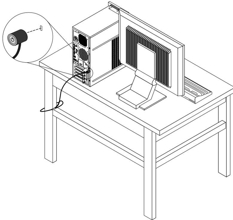
Figure 9. Integrated cable lock
