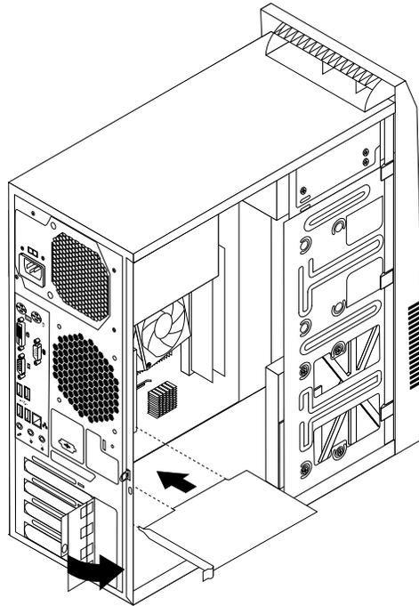
Figure 15. Installing a PCI card
