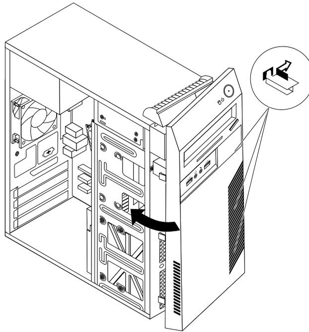
Figure 12. Reinstalling the front bezel
