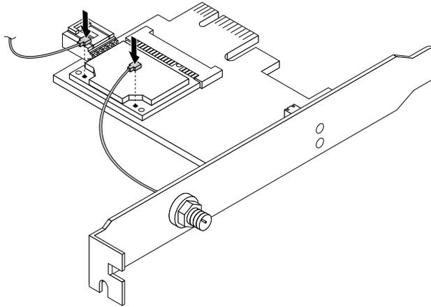
Figure 41. Installing the WiFi antenna cables
