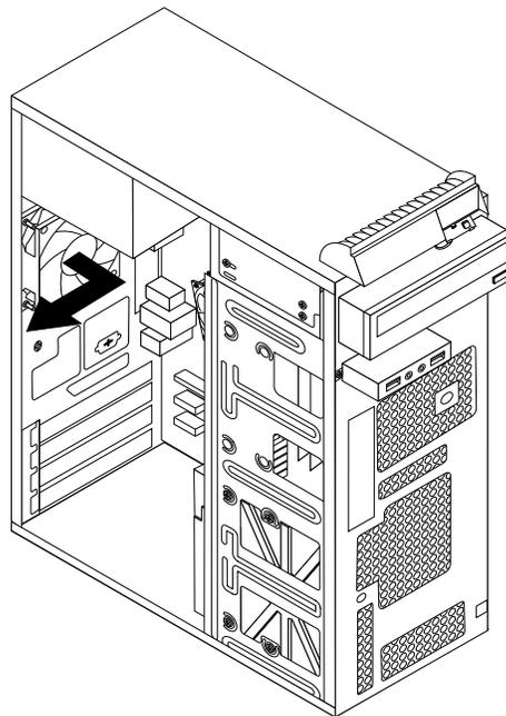
*Figure 33. Removing the rear fan assembly*
