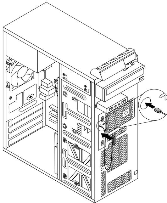
Figure 46. Installing the front WiFi antenna
