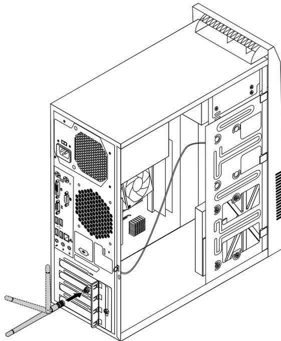
Figure 43. Installing the rear WiFi antenna
