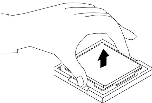
Figure 27. Removing the microprocessor
