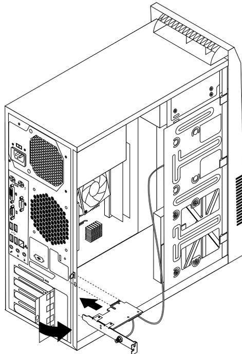
Figure 42. Installing the WiFi adapter card
