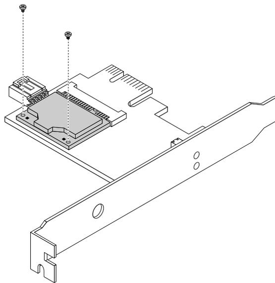
*Figure 38. Removing the screws that secure the WiFi card module*
