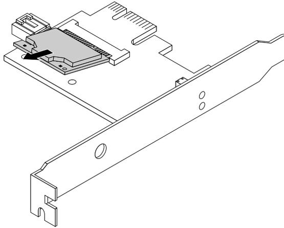
*Figure 39. Removing the WiFi card module*
