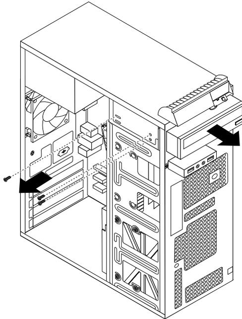
Figure 19. Removing the optical drive
