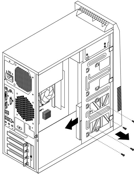
Figure 30. Removing the hard disk drive
