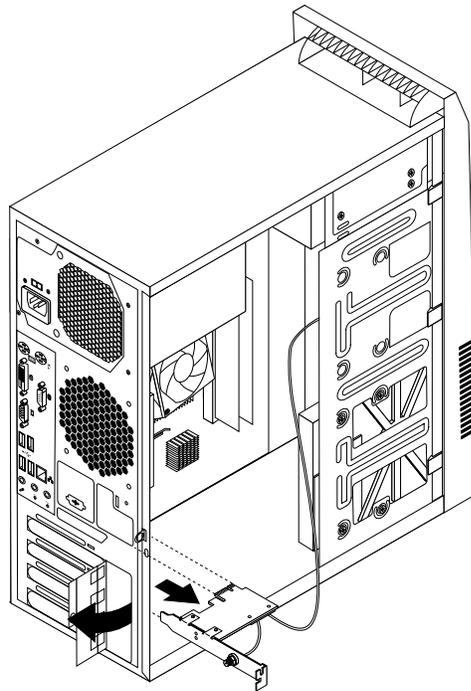
Figure 36. Removing the WiFi adapter card
