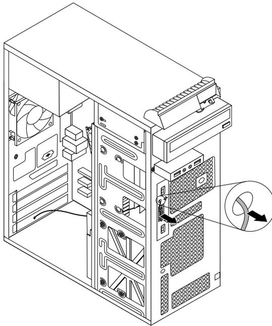
Figure 47. Removing the front WiFi antenna
