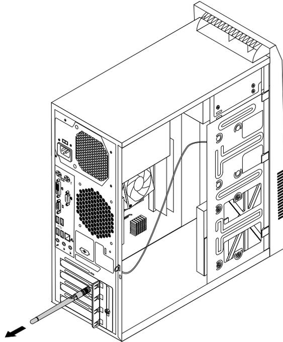
Figure 44. Removing the rear WiFi antenna
