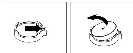
Figure 22. Removing the old battery
