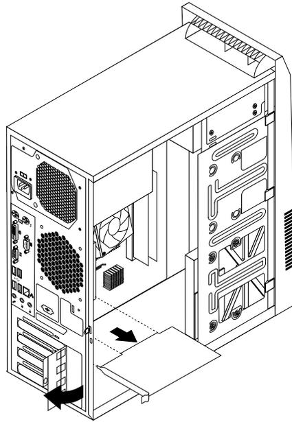
Figure 14. Removing the PCI card
