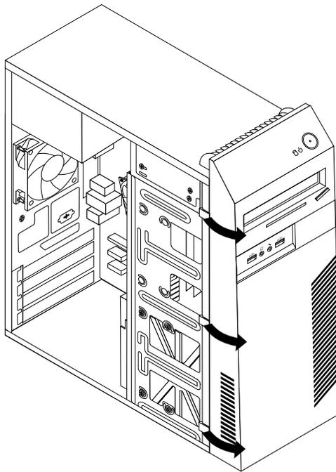
*Figure 11. Removing the front bezel*
