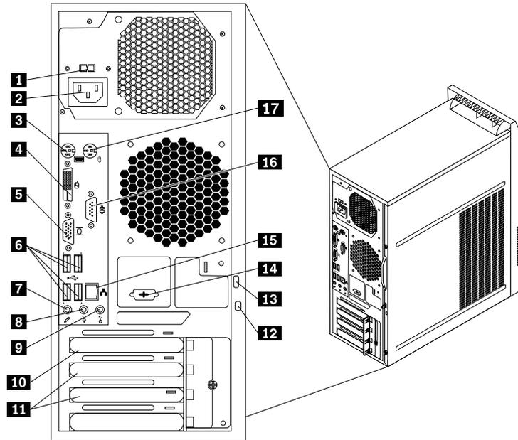
Figure 2. Rear connector locations
