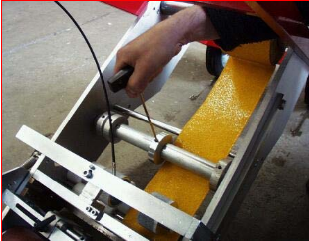
Figure 4: Adjustment of the upper tape guide rolls
