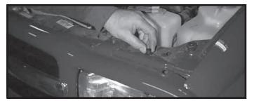
1. Remove grill by opening hood and removing plastic push fasteners from top of grill.
