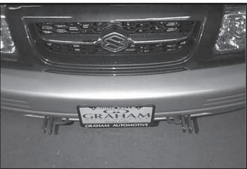
**10.** Install crossmember with 1/2" x 1-1/2" bolts, 1/2" lockwashers, and 1/2" hex nuts. (shims are included for crossmember if needed)
