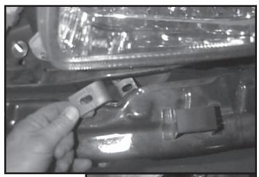
8. Remove top bumper bolt on each side and install brace with 8mm x 1.25 x 25mm bolt, 8mm lockwasher, and 8mm fender washer. Secure bottom of brace to frame mount using 3/8" x 1-1/4" bolt, 3/8" lockwasher,3/8" flatwasher, and 3/8" hex nut. We require that "L@CTITE" Blue" be used on all bolts.
