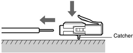
With the catcher facing down, press and hold the plug down against a flat surface and remove the cords from plug.
