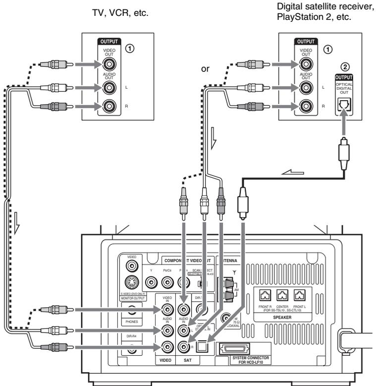
Connect the AUDIO OUT (L/R) jacks (①) to the VIDEO or SAT AUDIO IN (L/R) jacks of this subwoofer with audio cords (not supplied). If your TV does not have the AUDIO OUT (L/R) jacks, you cannot output the TV sound from the speakers of this subwoofer. If your TV has an OPTICAL DIGITAL OUT jack (②), connect to the SAT OPTICAL DIGITAL IN jack of this subwoofer using an optical digital cord (not supplied).
