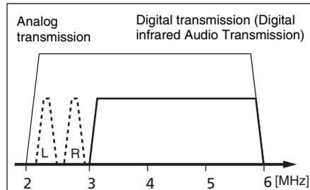
Fig. 1 Signal spectrum for digital infrared audio transmission
