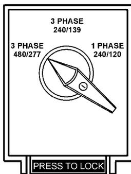
**Figure 27. Voltage Selector Switch 480/277V
