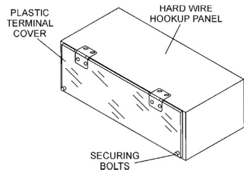
**Figure 12. Plastic Face Plate (Output Terminal Lugs)**
