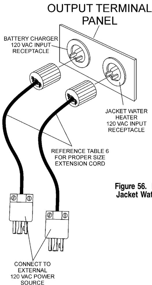
Figure 56. DCA-45SIU2 Battery Charger & Jacket Water Heater Power Connections
