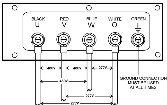
**Figure 28. Output Terminal Lugs
