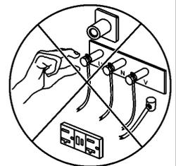
Backfeed to a utility system can cause **electrocution** and or property damage. **DO NOT** connect to any building's electrical system except through an approved device or after building main switch is opened. **ALWAYS** have a licensed electrician perform the installation
