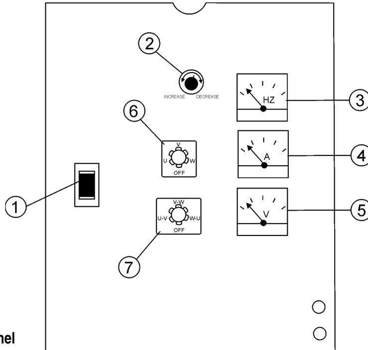
Figure 6. Generator Control Panel
