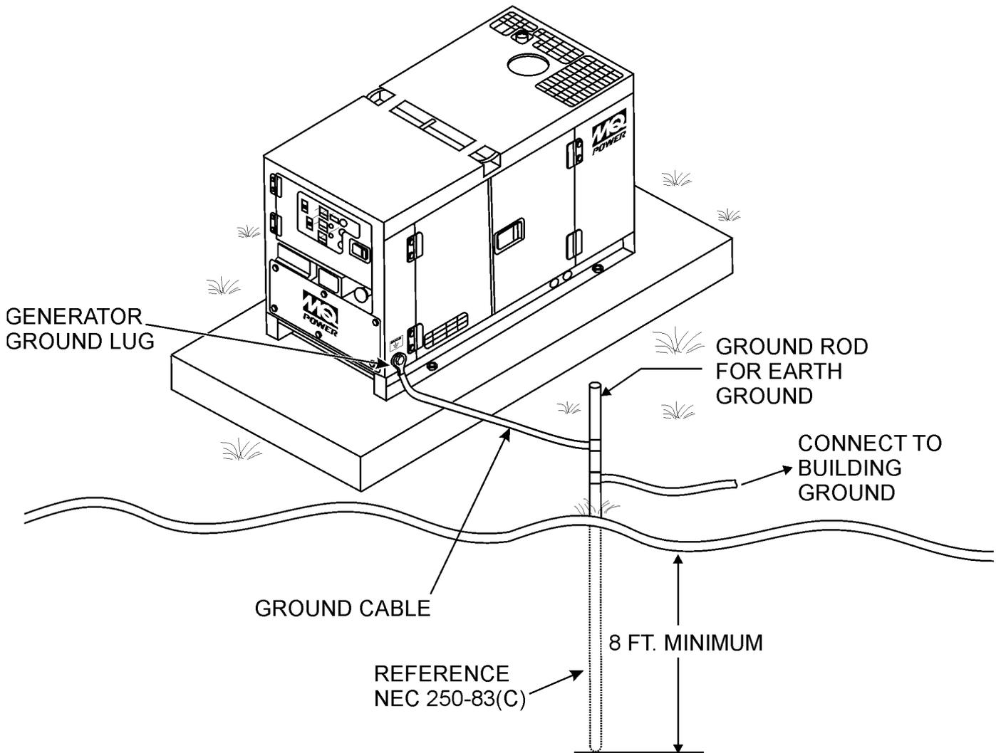
Figure 4. Typical Generator Grounding Application
