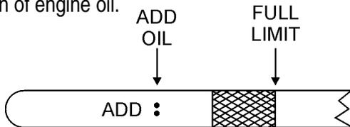
Figure 31. Engine Oil Dipstick
