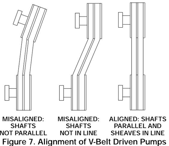
Tighten the belts in accordance with the belt manufacturer's instructions. If the belts are too loose, they will slip; if the belts are too tight, there will be excessive power loss and possible bearing failure.
