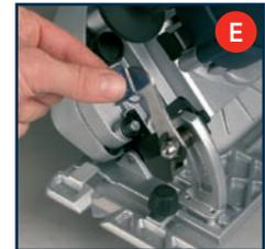
**Note.** Always make a trial cut in a scrap piece of material along a guideline to determine how much you should offset the blade from the guideline to make an accurate cut.
