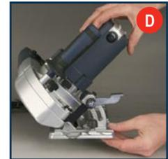
3. Tilt the body of the saw until the required angle is reached (Fig. D) using the bevel scale (7) as a guide.
