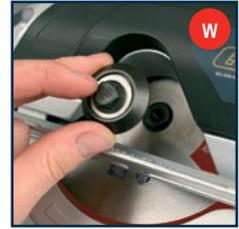
**WARNING.** The direction in which the blade rotates has to be the same as the direction of the arrow marked on the housing (26).
