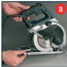
3. Hold the base plate flat against the edge of the work piece and lift the body of the saw until the blade is at the
