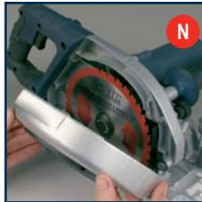
5. Dispose of the swarf and chips and wipe the collection chamber clean.
