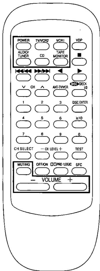
To turn the power of the amplifier ON/OFF
