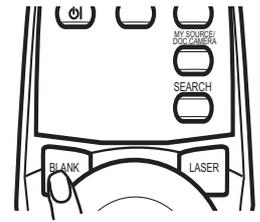
**⚠ CAUTION** ► If you wish to have a blank screen while the projector's lamp is on, use the BLANK function above. Any other method of blocking the projection light, such as attaching something to the lens or placing something in front of the lens, may cause the damage to the projector.
