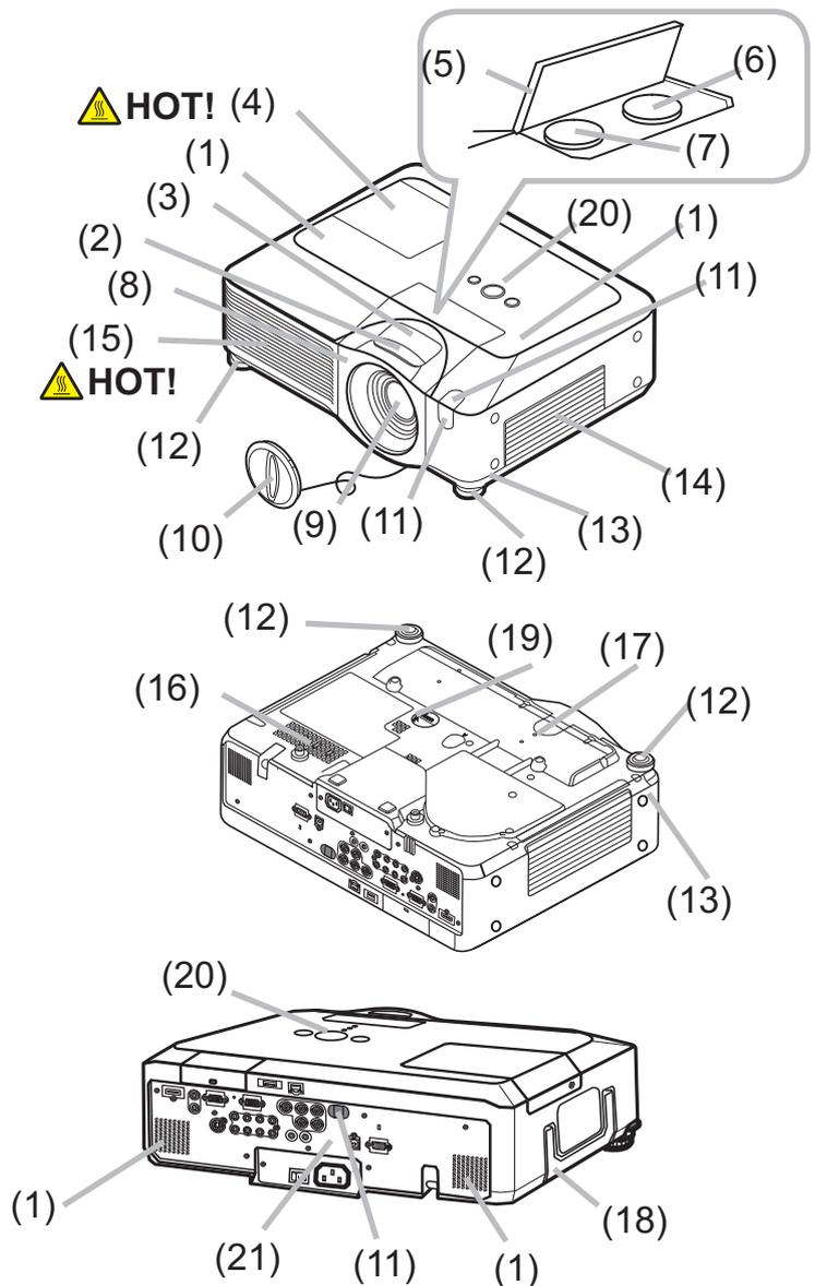
**⚠️ WARNING ►HOT!** : Do not touch around the lamp cover and the exhaust vents during use or just after use, since it is too hot.
