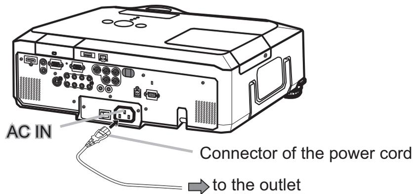
**⚠ WARNING** ▶ Please use extra caution when connecting the power cord, as incorrect or faulty connections may result in fire and/or electrical shock.
