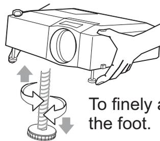
To finely adjust, twist the foot.
