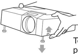
To loose an elevator foot, pull up the elevator knob on the same side as it.
