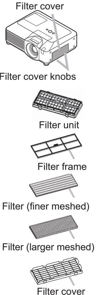
**⚠ WARNING** ► Before taking care of the air filter, make sure the power cable is not plugged in, then allow the projector to cool sufficiently.
