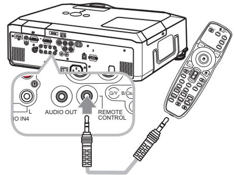
**NOTE** • To connect the remote control with the projector, use an audio cable with 3.5 diameter stereo mini plugs.
