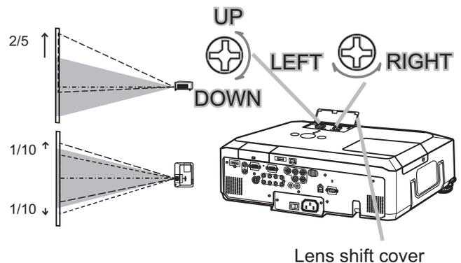
**NOTE** • When the vertical lens shift is adjusted, it is recommended to shift the picture upward.
