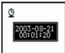
Then, using the NEXT/PREV buttons, adjust the numbers to correspond to the correct date. Press MENU to exit this sub-menu
