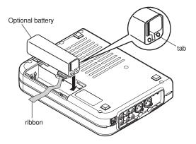
Install the battery with tab as shown and over the ribbon for easy battery removal.
