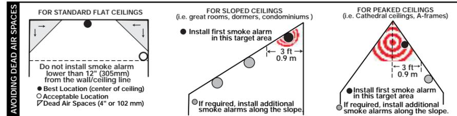
**"Dead air" spaces may prevent smoke from reaching the smoke alarm. To avoid dead air spaces, follow the installation recommendations below.**
