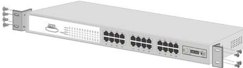
*Figure 6. Attach mounting brackets with screws*
