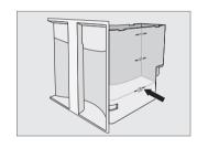
Fill the water container with lukewarm water up to the ///\\ symbol and add 1 sachet of the Original Miele cleaning agent for milk pipework. Push the water container back into the machine.
