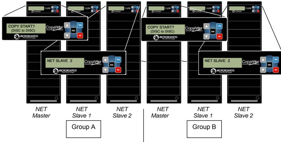
This can be done in any combination of towers. However, you must set the Master/Slave configurations starting with the last master you want to set, following the tower chain from the end to the beginning.
