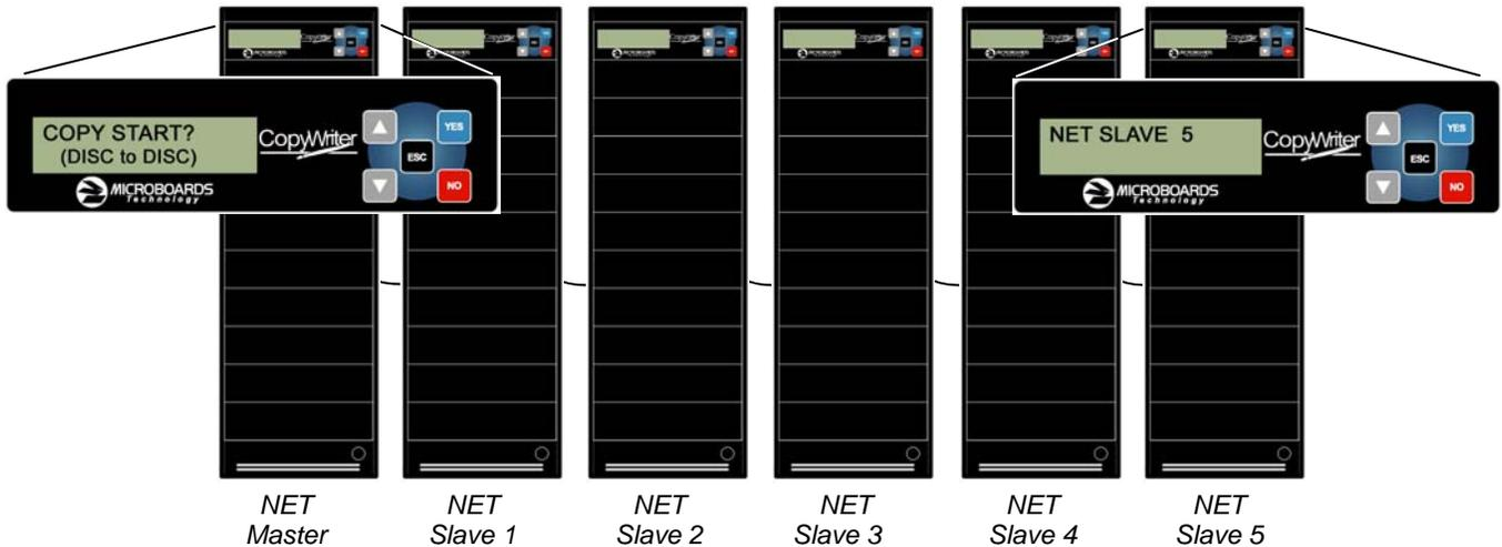
The result with a six-tower configuration is shown above. Only the reader and hard drive on the NET Master will be available as source drives.
