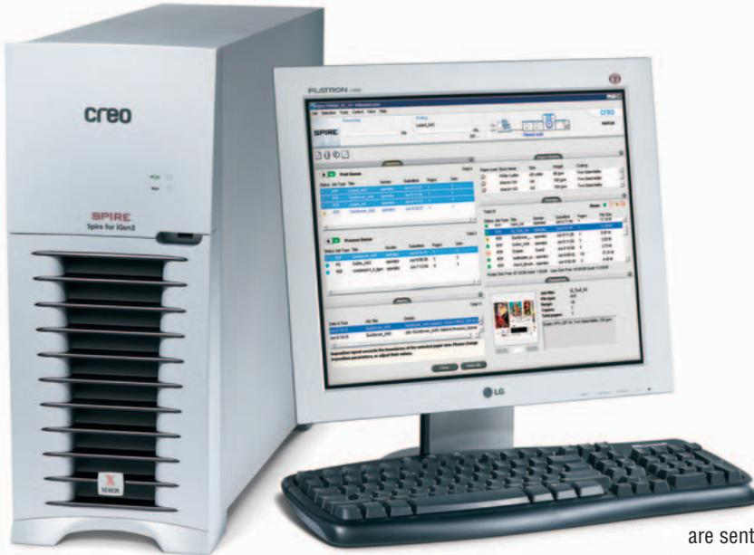
To boost productivity, Automatic Picture Replacement (APR), a powerful feature exclusive to Creo Color Servers, allows operators to work with low-resolution images before jobs are sent to print. The high-resolution images are held at the server and replaced on-the-fly at print time, saving both RIP time and disk space.
