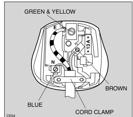
The plug moulded onto the lead incorporates a 13amp BSI362 fuse. Only ASTA or BSI fuses should be used.
