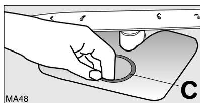
7. Put the flat filter (C) back in the base of the washing compartment.
