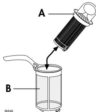
3. Turn the handle about 1/4 a turn anticlockwise and remove.
