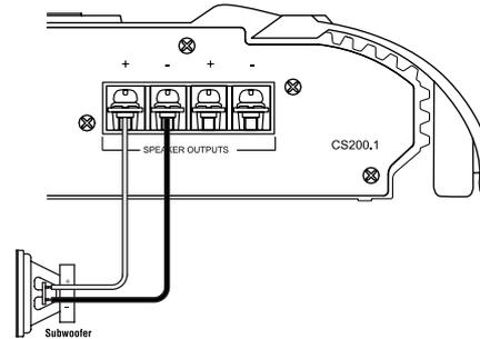
**Figure 3.** CS subwoofer amplifier with one woofer connection.
