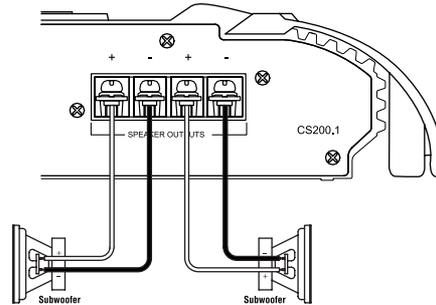
**Figure 2.** CS subwoofer amplifier with two woofer connections.
