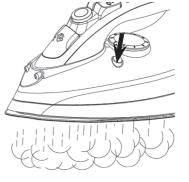
When Self-Cleaning is complete, release the Self-Clean button. Rest your iron on its heel rest and allow to fully cool down. Wipe the soleplate with a cold damp cloth. and store it safely.
