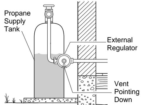
Figure 16 - External Regulator with Vent Pointing Down
