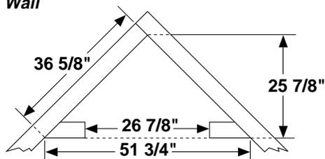
Figure 9 - Rough Opening for Installing in Corner
