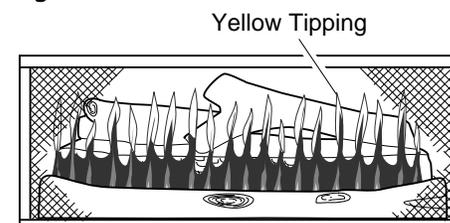
**Figure 33 - Incorrect Burner Flame Pattern**
