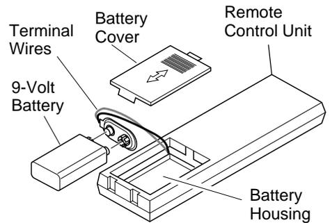
**Figure 25 - Installing Battery in Hand-Held Remote Control Unit**
