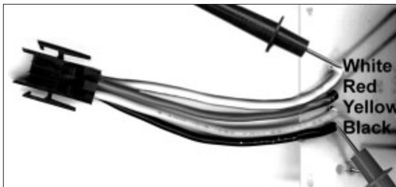
**STEP 5. CHECK THE PC BOARD.** Test for 24 VAC between the black PC board wire connection and ground.
