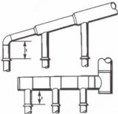
EXAMPLE: To combine two 6" vents with an 8" vent, the area of a combined vent should be one half area of two 6 inch vents (14 + 14) plus area of 8 inch vent (50) or 78 sq. inches. Referring to chart, 78 sq. inches require 10" diameter vent.
