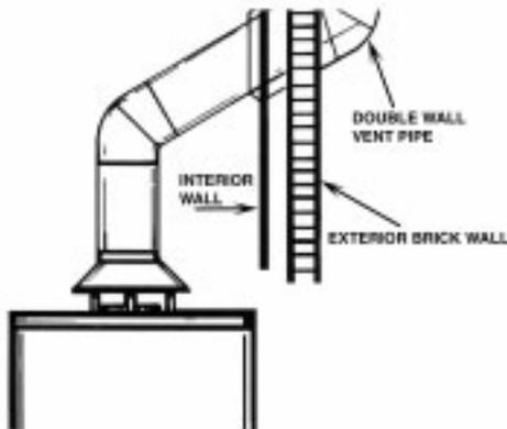
The vent pipe should be extended to meet local codes
