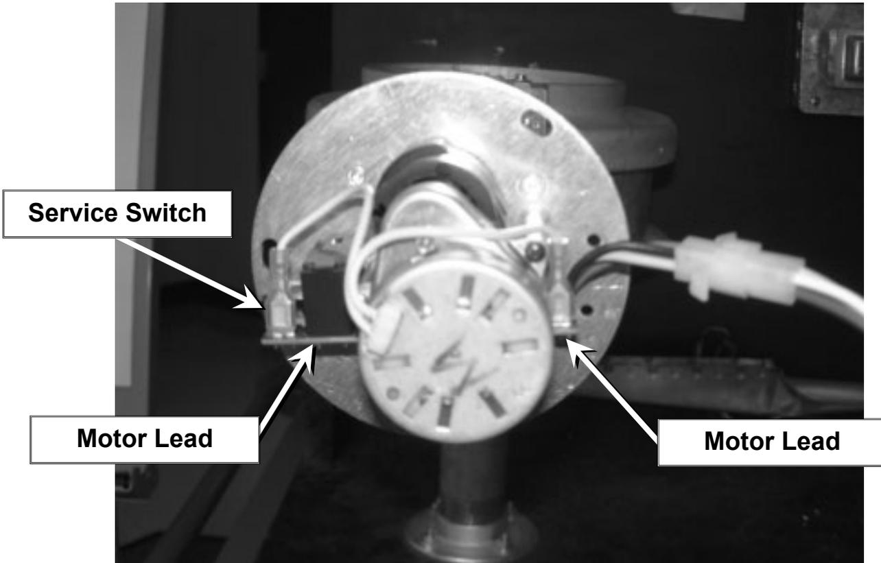
**STEP 6. PC BOARD/MOTOR TEST.** Check for 24 VAC between the two motor lead terminals of the PC board. Disconnect the wires for this test.
