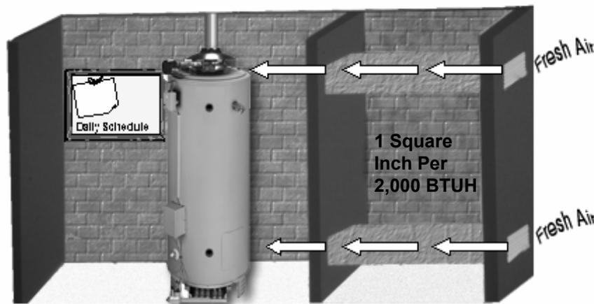
When the heater is installed in an interior room with no roof access for vertical ducts, horizontal make-up air ducts should be installed. When using horizontal ducts, two openings are required - one within 12 inches of the top of the enclosure and one within twelve inches of the bottom of the enclosure. Each opening shall have a free area of not less than 1 square inch per 2000 BTUH of the total input of all appliances within the enclosure.
