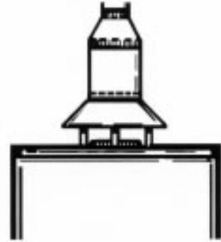
3. In some cases it may be necessary to run a vent larger than the draft diverter outlet.
