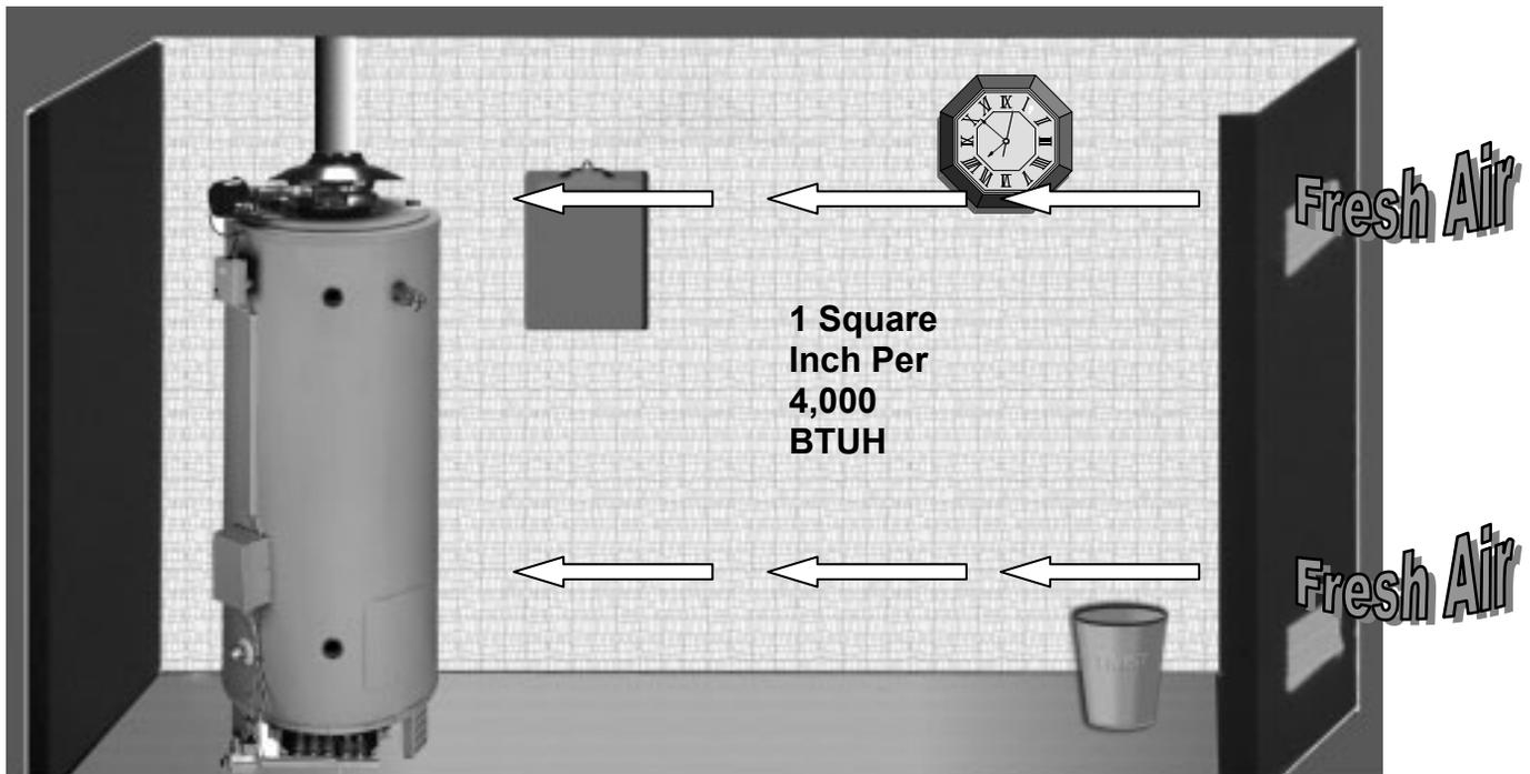
A fresh supply of make-up air for combustion can be supplied to the heater through make-up air ducts which directly communicate with the out of doors. Two openings are required - one within 12 inches of the top of the enclosure and one within twelve inches of the bottom of the enclosure. Each opening shall have a free area of not less than 1 square inch per 4000 BTUH of the total input of all appliances within the enclosure.
