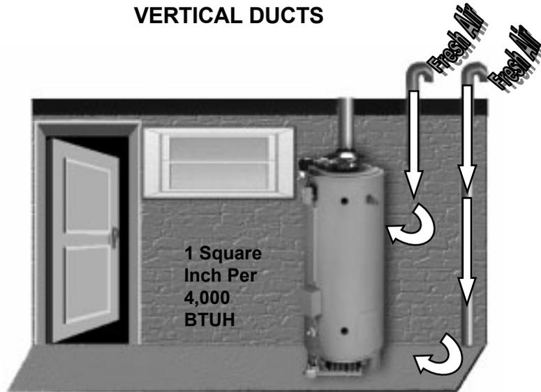
Often it is more practical to install vertical make-up air ducts to the out doors. Again, two openings are required - one within 12 inches of the top of the enclosure and one within twelve inches of the bottom of the enclosure. Each opening shall have a free area of not less than 1 square inch per 4000 BTUH of the total input of all appliances within the enclosure.
