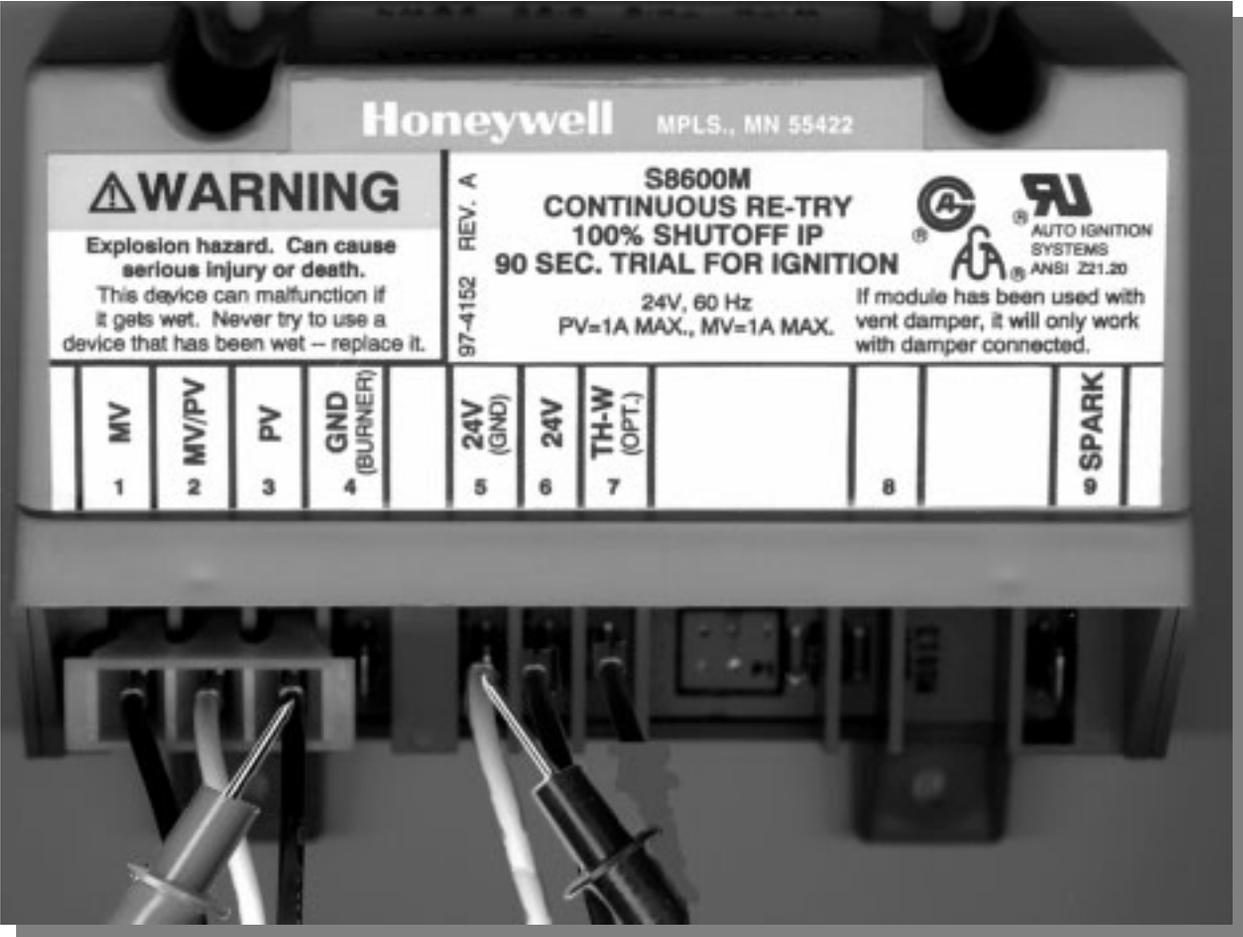
**STEP 12. IID MODULE TEST (Power to the Pilot Valve).** Using a multimeter, test for 24 VAC between terminal PV and 24V (GND) on the IID during the 90 second trial for ignition.
