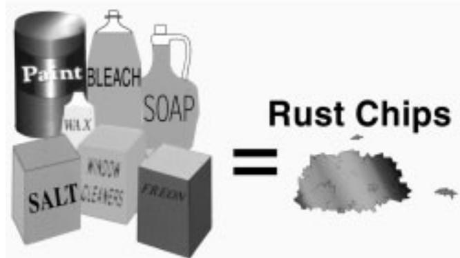
Along with adequate make-up air, the quality of the air is important. Contaminants in combustion air can lead to premature heater failure. Vapors from bleaches, soaps, waxes, salts, etc. are drawn into the combustion chamber with the make-up air and, once fired, mix with water vapor in the gases to form extremely corrosive hydrochloric or hydrofluoric acid and other corrosive byproducts.
