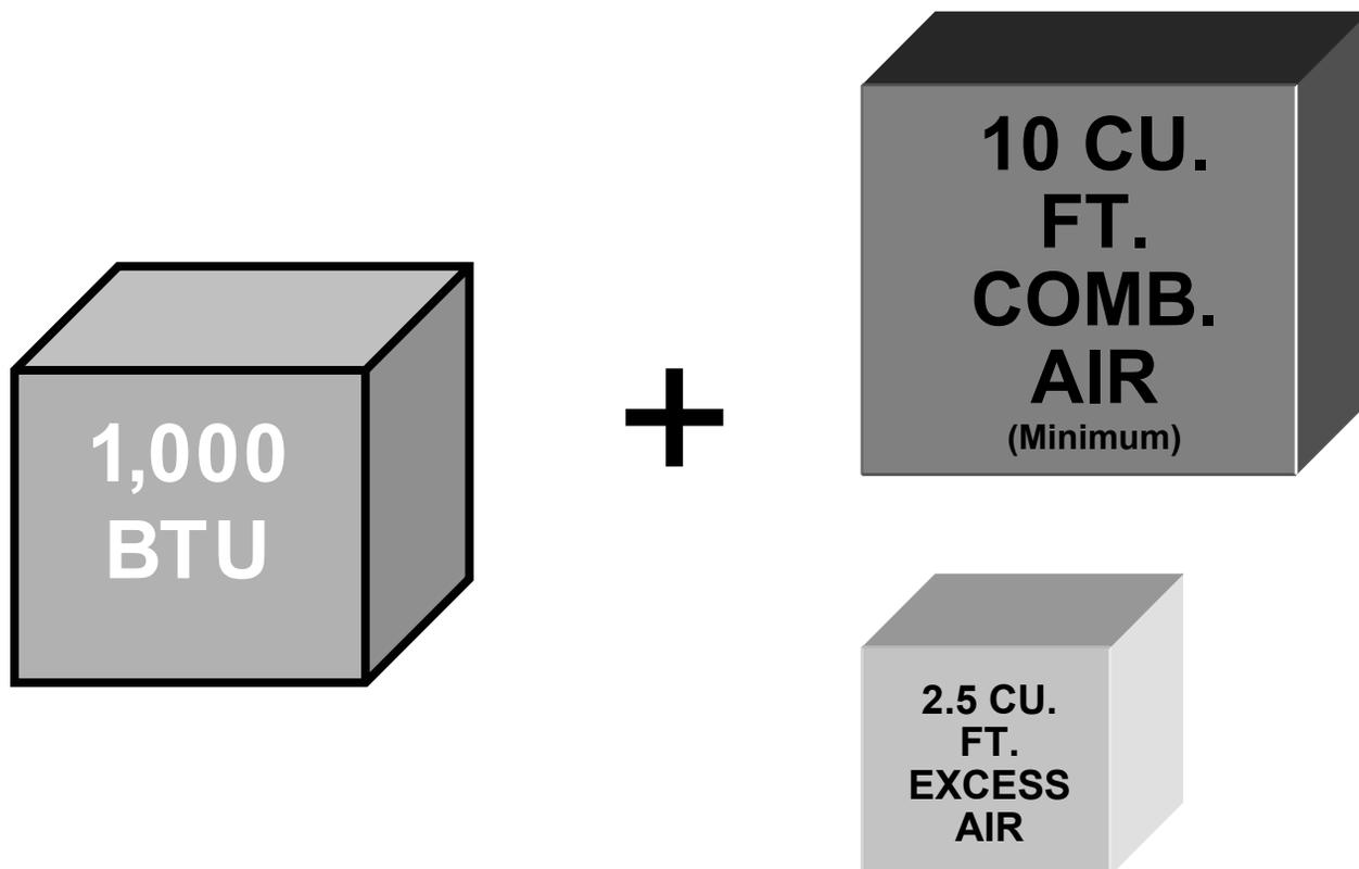
Stoichiometric or theoretical complete combustion requires 10 cubic feet of air per 1000 BTUH input of the gas input. The National Fuel Gas Code also recommends an additional 2.5 cu.ft. of "excess" air. This 12.5 cu.ft minimum supply air per 1000 BTUH input applies to natural and propane gas models.
