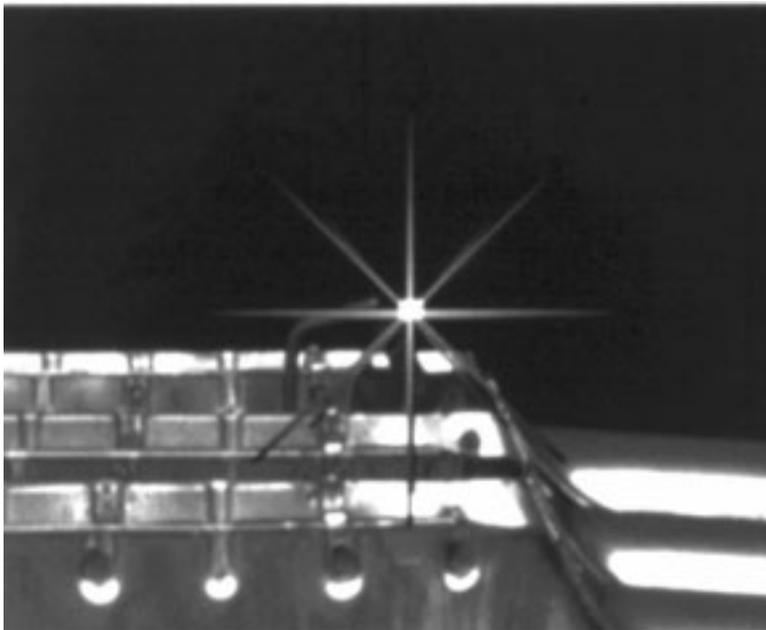
**STEP 13. PILOT SPARK TEST.** Visually check for spark at the pilot assembly.
