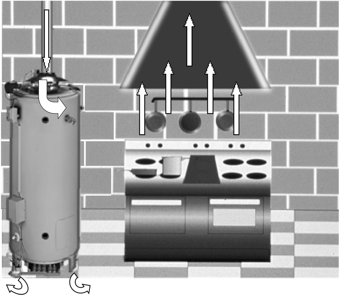
Insufficient make-up air is a major cause of combustion problems. One common example is in a restaurant installation where exhaust vent equipment was not considered in sizing make-up air requirements. This may result in air being backdrafted by the restaurant exhaust equipment through the heater causing flue gas spillage, flame roll out, improper combustion, inconsistent pilot operation, and/or erratic heater shut down.
