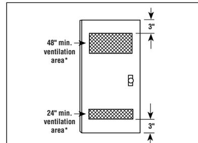
\*For closet installation with a door, the minimum ventilation openings in the top and bottom of the door are required. Louvered doors with equivalent ventilation openings are acceptable.
