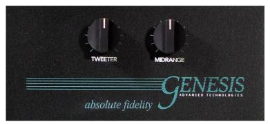
clockwise will increase the level of the front tweeter. Use this control if you need a bit more treble or to increase the apparent space of the soundstage. Start with this control at the 12 o'clock position. There is about a one dB range for this control. The 12 o'clock straight up position is nominal for all controls.
