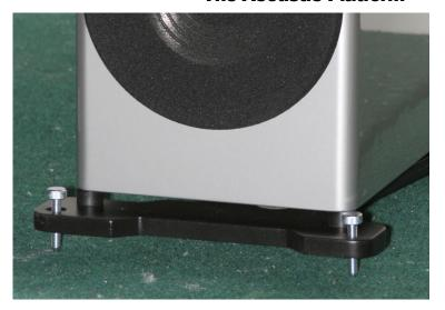
The G5 sits on a suspension system designed to allow the loudspeaker to perform at its optimum. It consists of three elements – neoprene decouplers, a tuned skeletal frame, and stainless steel spikes. The system holds the loudspeaker firmly, and yet isolates it from the floor on which it sits.
