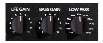
The knob on the middle of the lower row of knobs marked "Bass Gain" controls the volume of the built-in bass servo amplifier. Begin with this control at 6 (the 12 o'clock position). Adjusting the gain higher will make the loudspeaker sound "fuller" and more bass-heavy.
