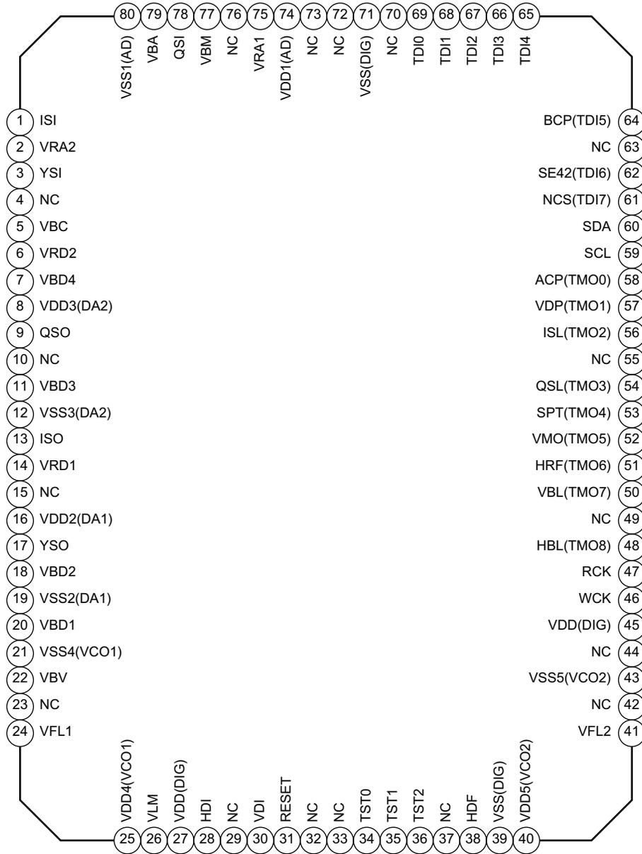
Fig. 5-2 Pin function of TC9097F (QFP 80 pin)
