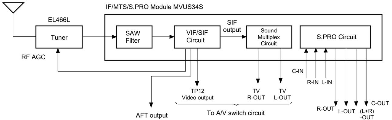
Fig. 2-1 Block diagram
