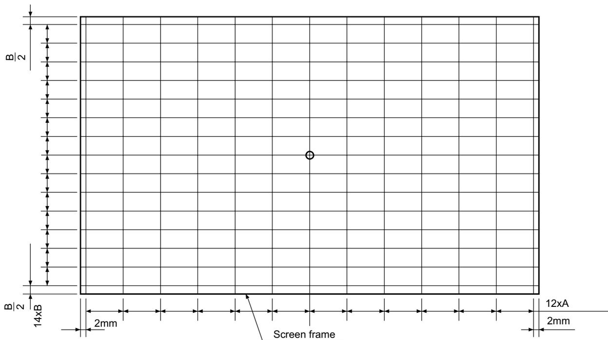
40 inches 16:9 Screen size: Horizontal 885mm x Vertical 498mm
