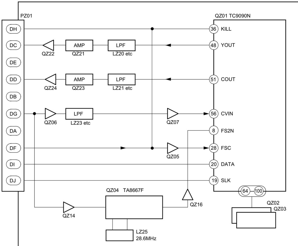
Fig. 7-1 3-dimension Y/C separator unit block diagram
