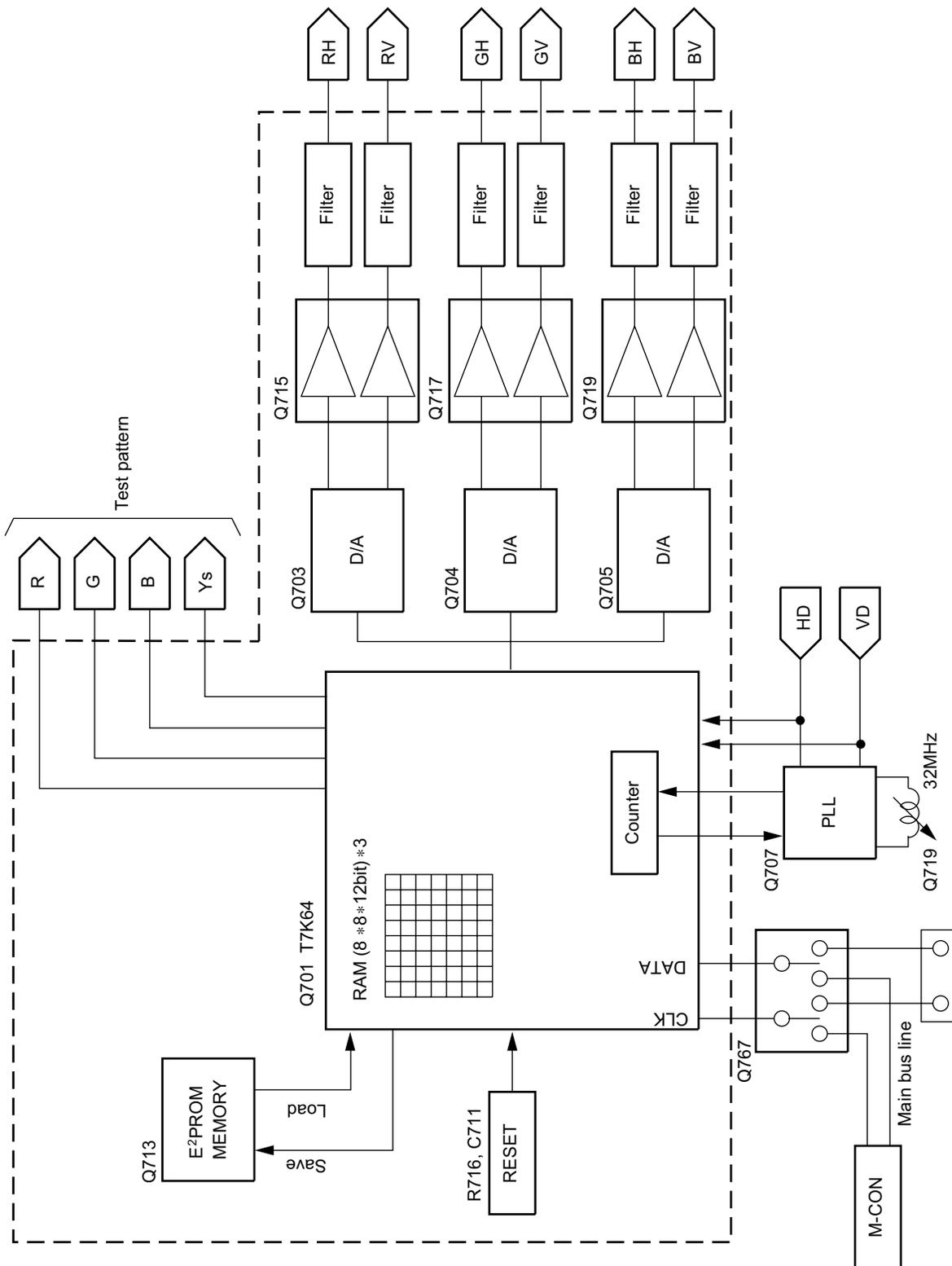
Fig. 11-1 Block diagram
