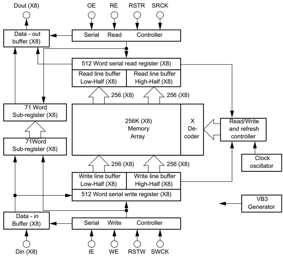
**Fig. 6-9 QY10/QY11 M518221-30ZS internal block diagram**
