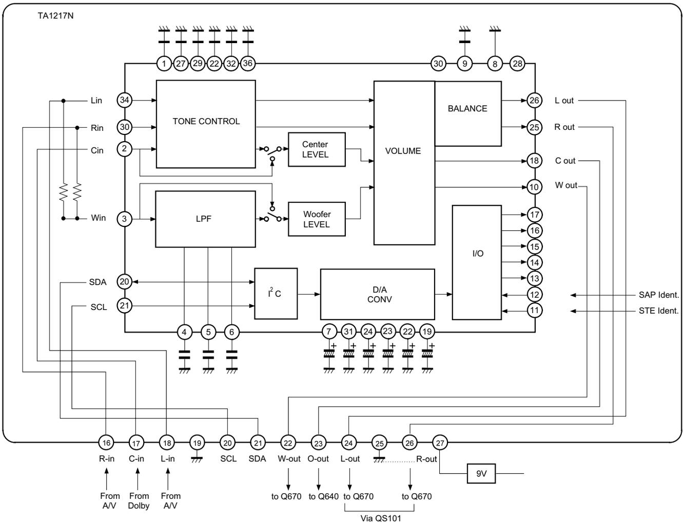
Fig. 2-3 A.PRO block diagram
