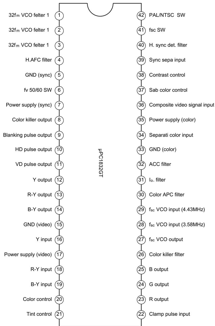
**Fig. 6-6 QY01 mPC1832GT pin layout**
