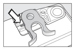
Using a screwdriver, remove spring clamp (9) from underneath the door and fit it on the opposite side.
