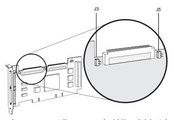
You might want to manually terminate the SCSI card if the Adaptec SCSI Card 39160 is connected to one or more external SCSI devices that are also connected to a SCSI card in another computer. The devices can be shared between the two computers if one SCSI card is terminated when it is powered off, while the computer with the other SCSI card is using the SCSI devices.
