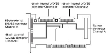
■ Internal Ultra2 and Ultra160 SCSI devices come from the factory with termination disabled and cannot be changed. Proper termination is provided by the terminator at the end of the internal LVD SCSI cable.
