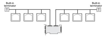
The following example shows LVD (Ultra160 and Ultra2) SCSI devices on Channel B and non-LVD SCSI devices on Channel A.
