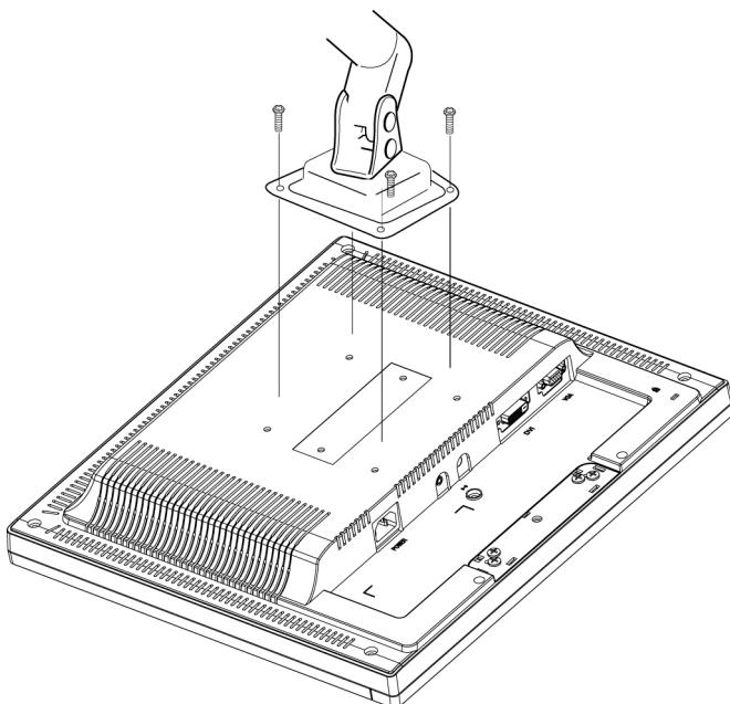
Follow these steps to finish installing the wall mounting arm:
