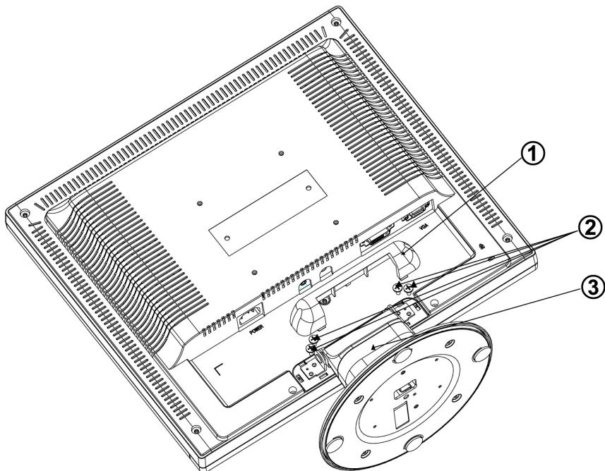
This monitor can be attached to a wall mounting arm you can purchase separately. Turn the power OFF then dis-connect the cables from the monitor before performing the procedure below. Lay the monitor face down on a soft surface.
