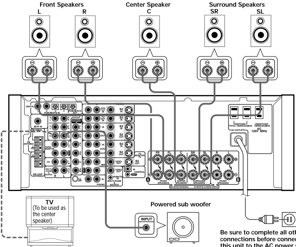
When using the speaker on your TV as the center speaker, connect the CENTER PREOUT jack on this unit to the audio input jack on your TV. In this case, the center speaker shown is unnecessary.
