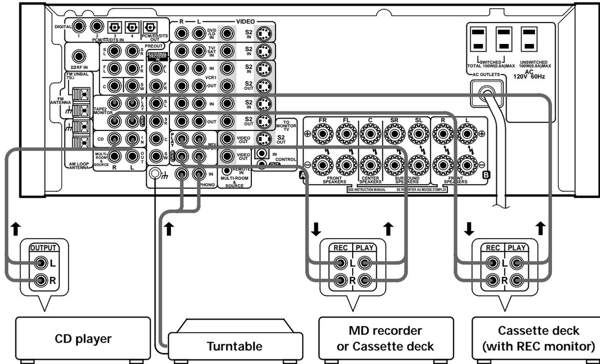
If your turntable has a ground wire, connect it to the SIGNAL GND terminal.
