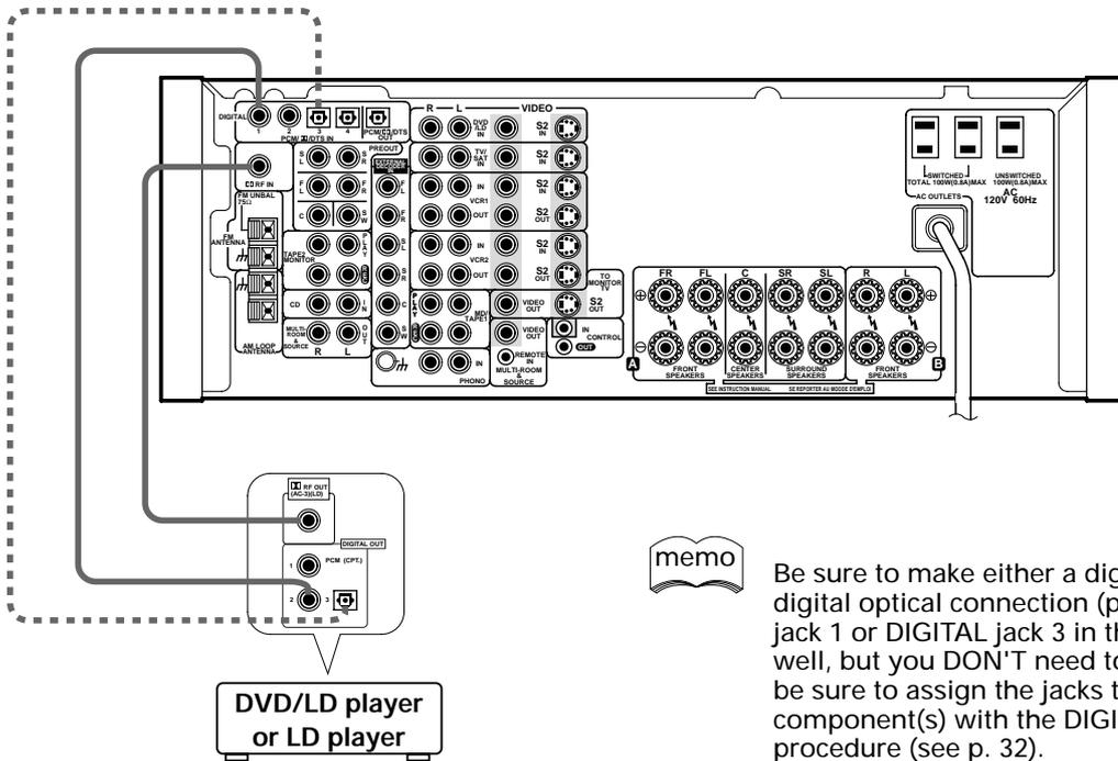
Be sure to make either a digital coaxial or digital optical connection (pictured as DIGITAL jack 1 or DIGITAL jack 3 in this diagram) as well, but you DON'T need to make both. Also, be sure to assign the jacks to the proper component(s) with the DIGITAL INPUT SELECT procedure (see p. 32).
