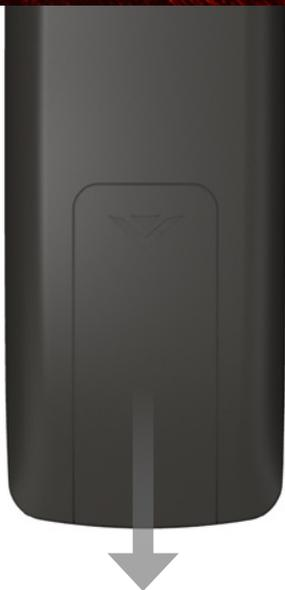
Remove the battery cover by pressing gently and sliding away from the remote.
