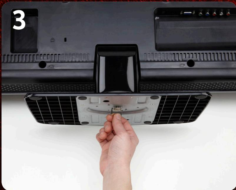
Turn the attached thumbscrew until it is completely tightened.
