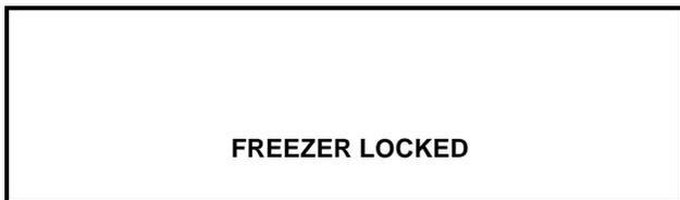
To restore the message that identified the reason for the hard lock, turn the power switch OFF for five seconds and then return the power switch to the ON position. The original message with the reason for the Hard Lock will be displayed.
