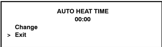
To set the AUTO HEAT TIME, touch the UP arrow symbol to move the arrow to "Change". Then touch the SEL symbol. The screen will display the time with the cursor under the hour position.
