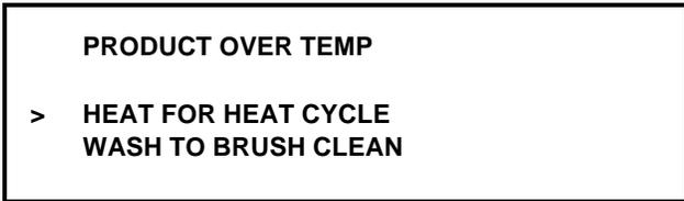
When one of these messages appears, automatic freezer operation cannot take place until the freezer is disassembled and brush cleaned, or has completed a heat treatment cycle.
