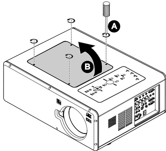
2. Loosen the two captive screws on the lamp module (A). Lift the module handle up as shown (B).
