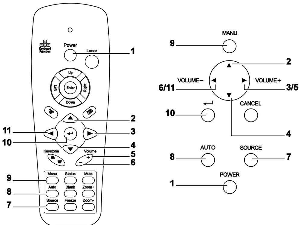
Some buttons on the projector have two functions. For example, item 6/11 on the projector functions as both the volume down button and as the left cursor key in OSD menus.
