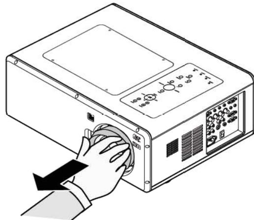
2. Push the LENS RELEASE button all the way in and rotate the lens counterclockwise.
