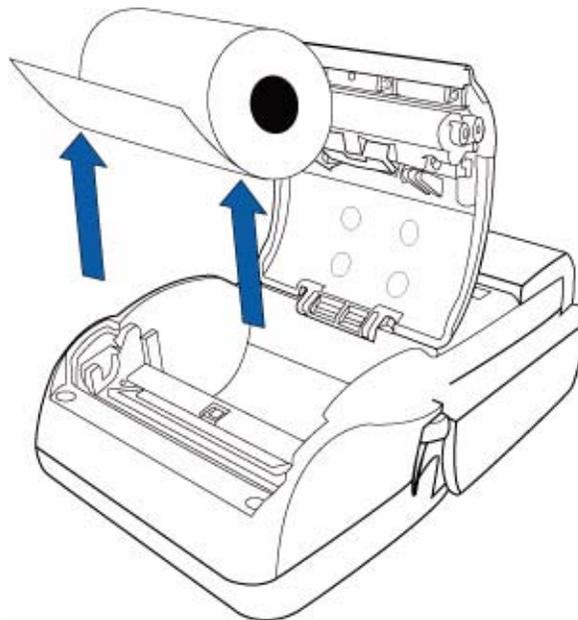
**Figure 10** Removing Partial Paper Roll
