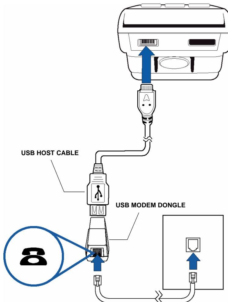
Figure 7 V<sup>x</sup>670 USB Modem Dongle Connection
