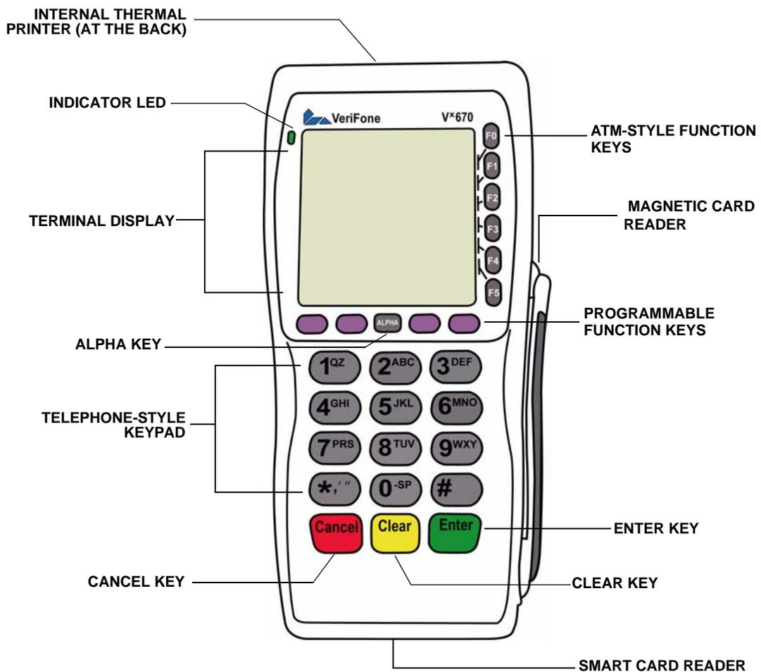
**Figure 2** V<sup>x</sup>670 Terminal Features (Front Panel)
