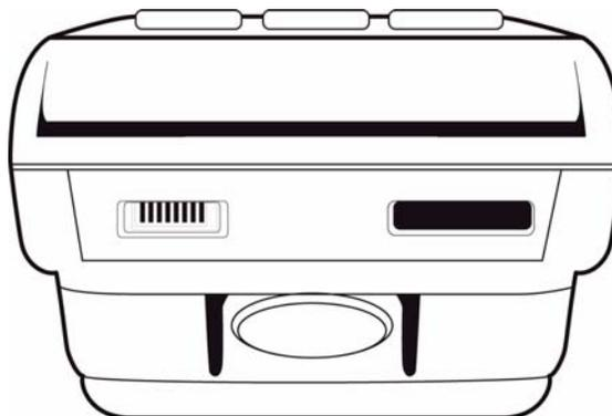
**Figure 3** The Vx670 Primary Port (Bottom View)
