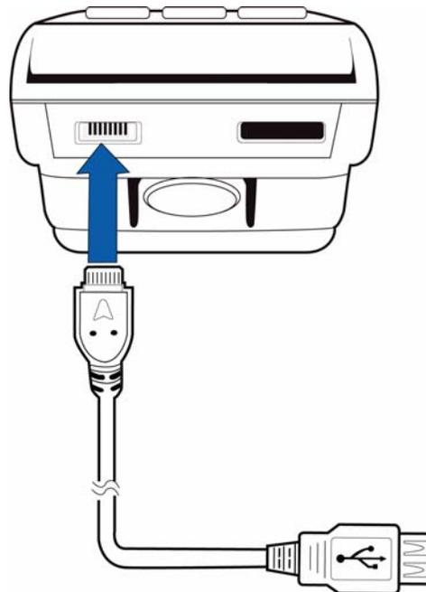
**Figure 5** USB Host Cable Connection to a V<sup>x</sup>670 Terminal
