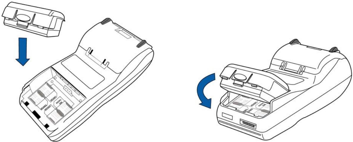
**Figure 17** Installing the Smart Battery
