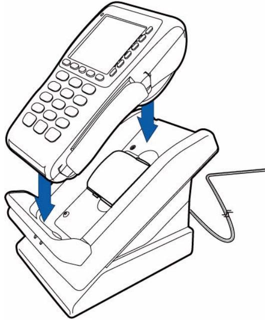
**Figure 26 Charging the Spare and Installed Battery Simultaneously**
