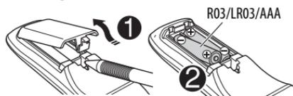
Insert the batteries into the remote controller by matching the polarity (+ and -) correctly.
