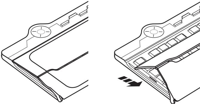
Lift and fold the dust cover to the open position.
