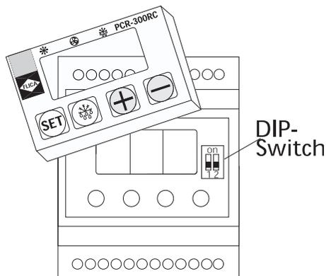
Carefully lift the housing cover off the side, using your fingers.
