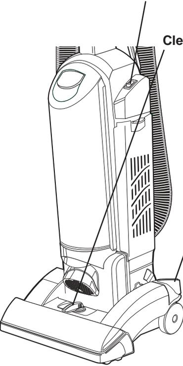
**Cleaner Height Setting.** An adjustment that raises or lowers the cleaner base to match the type of floor surface. With the cleaner cord unplugged, set the adjustment to lowest setting for maximum carpet cleaning. **If the cleaner is difficult to push, move adjustment to next highest setting until cleaner is comfortable to push.**
