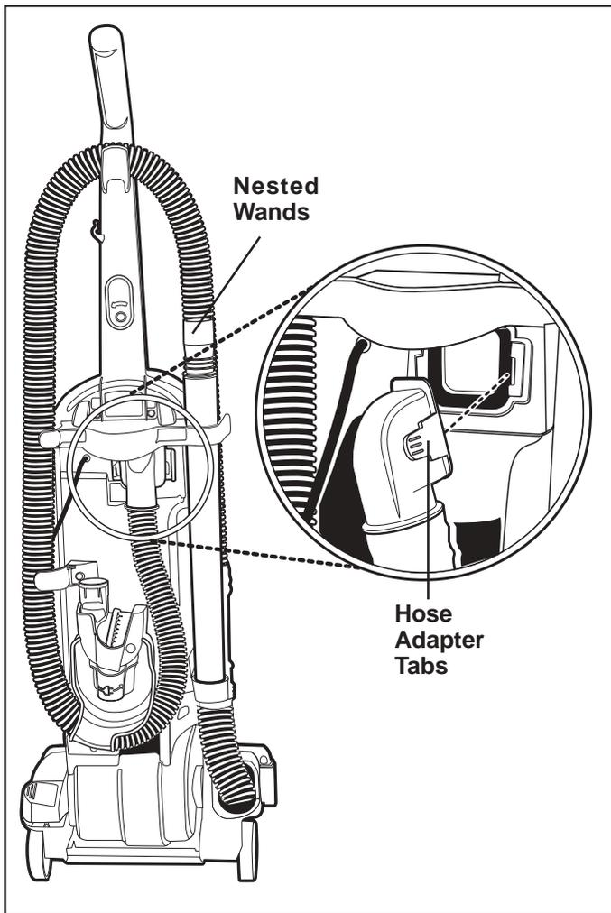
**NOTE:** Turn off the switch and unplug the electrical cord before clearing hose.
