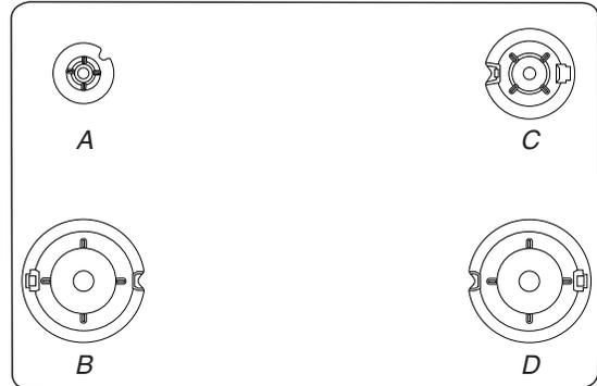
5. Replace the burner cap, making sure it is properly aligned with the burner base. The burner cap should not rock or wobble when properly aligned.
