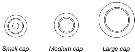
Burner caps should be level when properly positioned. If burner caps are not properly positioned, surface burners will not light. The burner cap should not rock or wobble when properly aligned.
