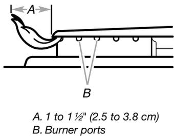
**Burner Ports:** Check burner flames occasionally for proper size and shape as shown in the previous illustration. A good flame is blue in color, not yellow. Keep this area free of soil, and do not allow spills, food, cleaning agents or any other material to enter the burner ports.
