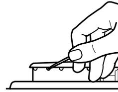
4. Replace the burner base. See the following illustration for burner positions.
