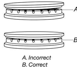
**IMPORTANT:** The bottom of the small and medium caps are different. Do not put the wrong size burner cap on the burner base.
