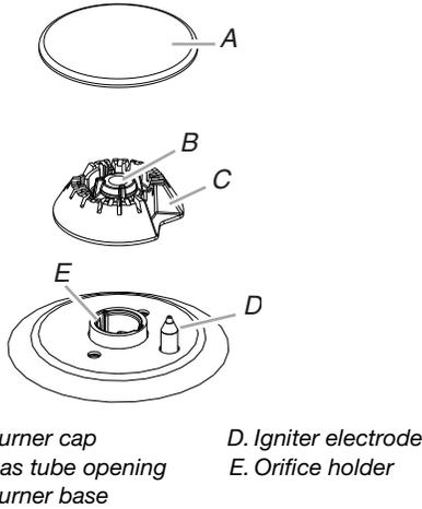
**Gas Tube Opening:** Gas must flow freely throughout the gas tube opening for the burner to light properly. Keep this area free of soil, and do not allow spills, food, cleaning agents or any other material to enter the gas tube opening. Keep spillovers out of the gas tube opening by always using a burner cap.
