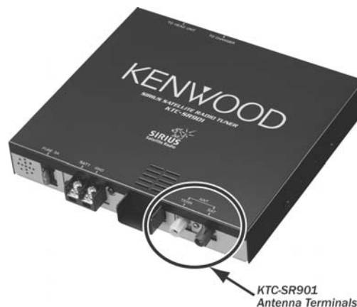
Figure 17: Connecting the Sirius receiver
