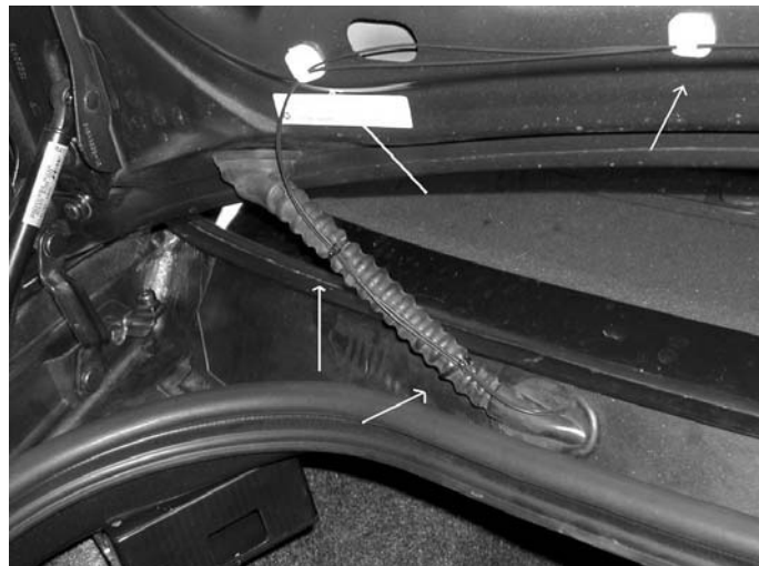
Figure 20: Attaching the cable to the cable channel
