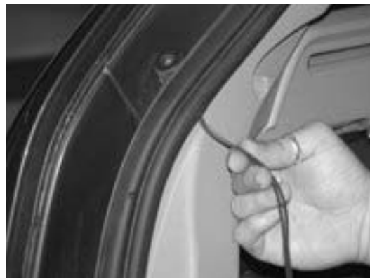
Figure 27: Hiding the cable under the rubber molding
