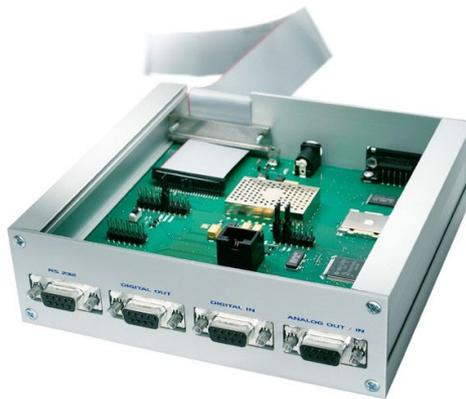
**Figure 4. Evaluation module for Nokia M2M ADK**
