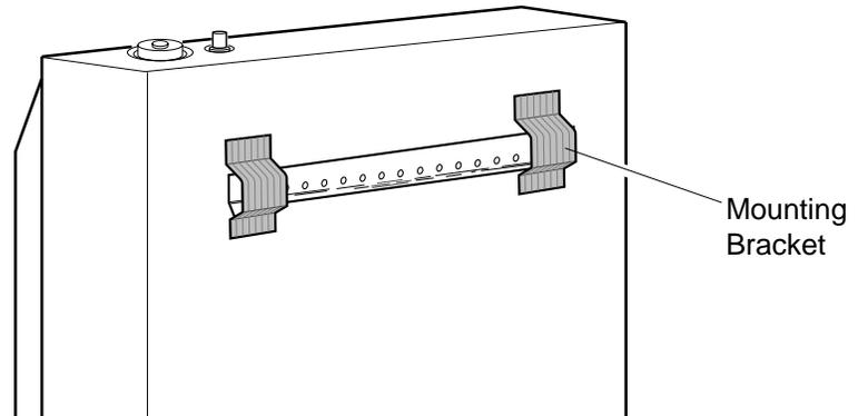
**Figure 6 - Mounting Bracket**
