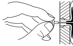
**Figure 10 - Popping Open Anchor Wings For Thin Walls**
