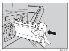
Remove the red sheet from the photo conductor unit and remove the two pieces of tape.
