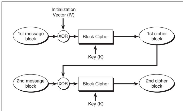
Figure 3-4 **Cipher-Block Chaining (CBC) Mode**
