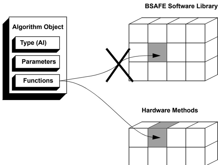
Figure 4-2 **Algorithm Object in a Hardware Implementation**
