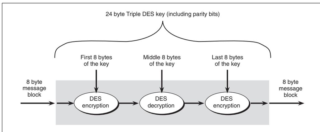
Figure 3-2 Triple DES Encryption as Implemented in Crypto-C
