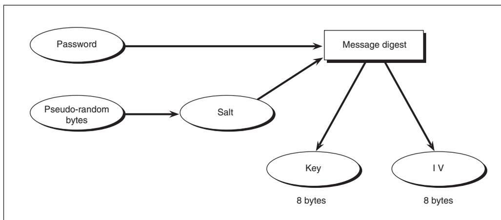
Figure 3-8 **DES Key and IV Generation for Password Based Encryption**
